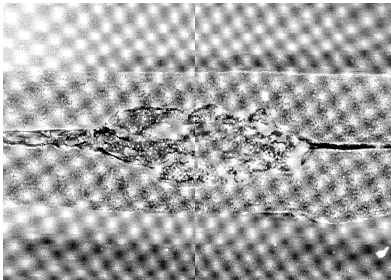
Fig. 2. Poor welding connection lug-substrate.
